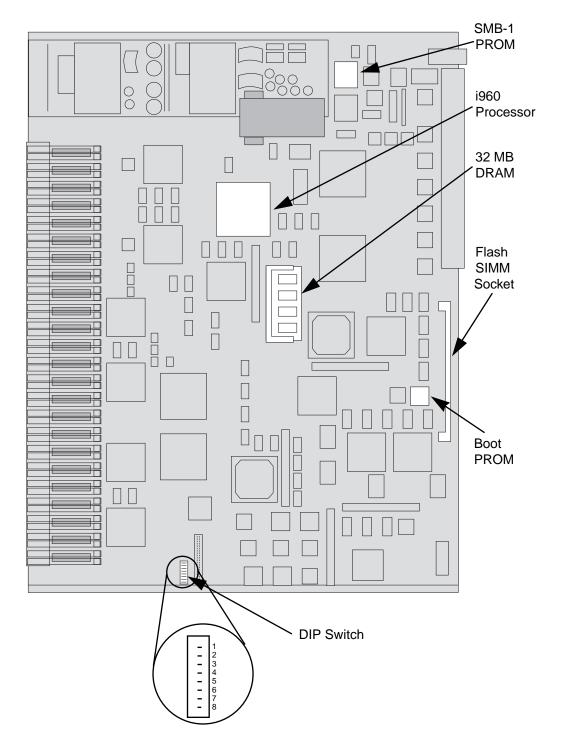
Figure 2-1. User-Accessible Components
